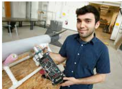
Aerospace student Atila Saadat holds an avionics bay, which will log the altitude of a rocket he is building with a team of UWindsor students.
